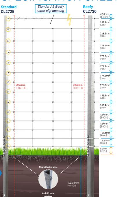
Designed specifically for all X fence 13/190 deer or boar fence patterns with one line of barbed, plain or electric above. Clips all lines.
