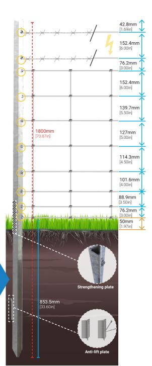
Entry level post suitable for most hinge jointed 8/80/15 & 30 stock fences. It can also be used for permanent electric fencing and rabbit fencing.
