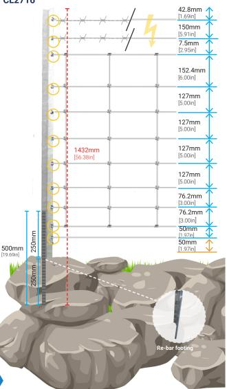
Specifically designed for installing over rocks or concrete. It is for use with 8/80 X fence stock fence mesh patterns but can also be used for permanent electric fencing, line wire, barbed wire or rabbit fencing.
