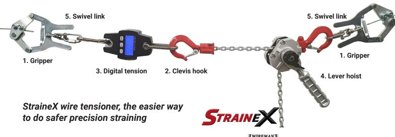
The Wireman StraineX wire tensioner kit is extremely simple and easy to use, ensuring full precision control. The lever hoist with the clevis hooks can be used with strainer boards to tension fabricated netting, when combined with Grippers it can strain both plain or barbed wire. Fast and easy to use and remove, clip on/off parts. A one tool must have for every fencer's toolbox.
