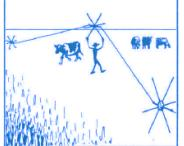
Lift Tumblewheels up vertically to allow stock and machinery to pass underneath wire.
