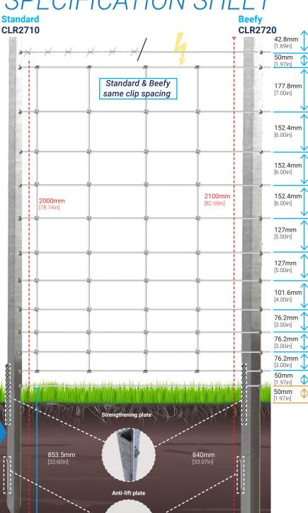
Specifically designed for railway boundaries although its added height makes it suitable for cattle/dog fencing also. We recommend using Beefys at slight change of direction or where there are pressure points on undulating ground. We also recommend using Beefys to strengthen adjoining paddock fences.
