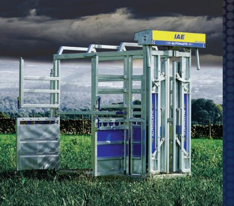
Where the need for access outweighs a squeeze requirement the A800 Full Access gives an incredibly robust, self-locking crush with excellent access to all areas of the cattle's body. 72 Acoustic Dampening Points (ADP) ensure a calm and quiet working environment, helping you to improve your throughput and complete routine handling tasks quicker.
