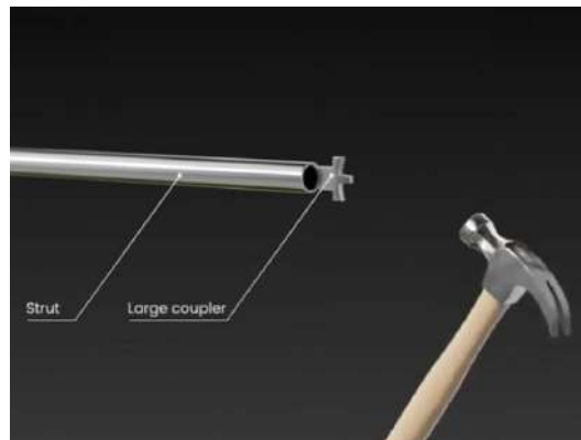
4. Hammer in the large coupler to bottom of the strut post.
